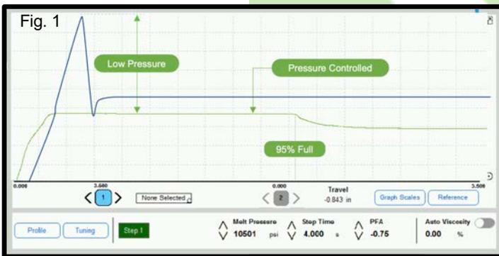
The Blue Curve™ represents plastic pressure during the conventional injection molding process, while The Green Curve™ represents that same plastic pressure with the iMFLUX process.
