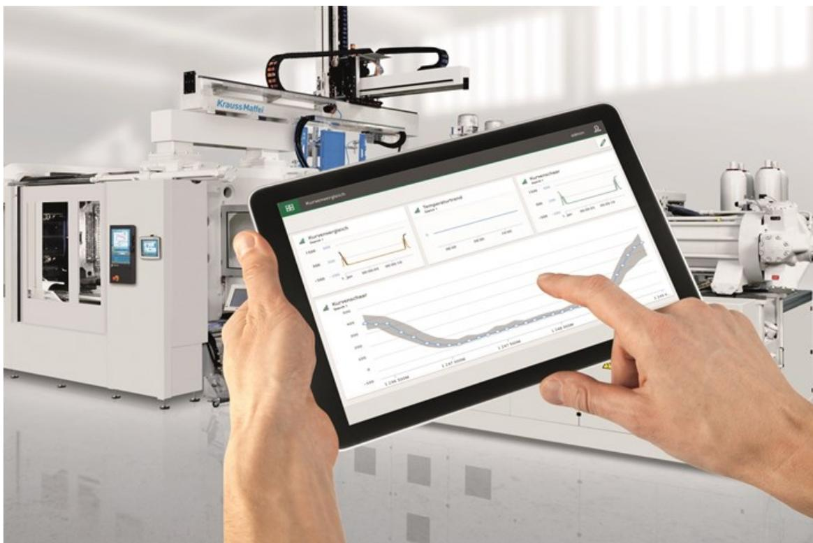
Artificial intelligence (AI) is increasingly a feature of Industry 4.0 digitization of molding operations. An example is KraussMaffei's new app to provide early warning of production anomalies. KM plans to extend real-time production monitoring to non-KM equipment.
