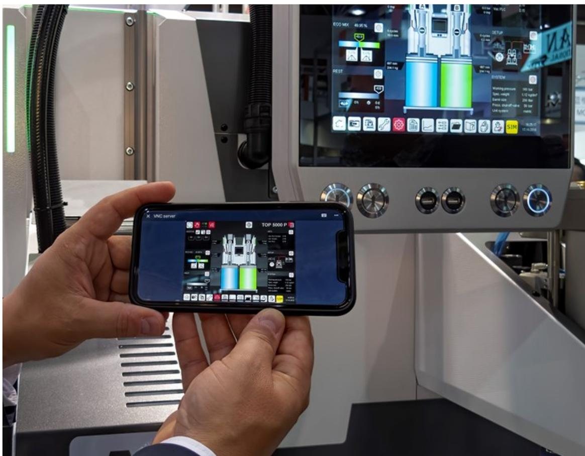
Elmet showed its new servo-driven TOP5000E LSR dosing system with web connectivity and remote monitoring/control via mobile devices.
